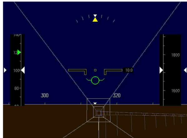
**Fig. 7.5.** *Effect of 10 degrees pitch with an inside-out frame of reference. In this frame of reference, the pitch angle is coupled to the vertical translation of the displayed scene which is much more compelling as the motion of the single aircraft symbol in the previous figure.*
