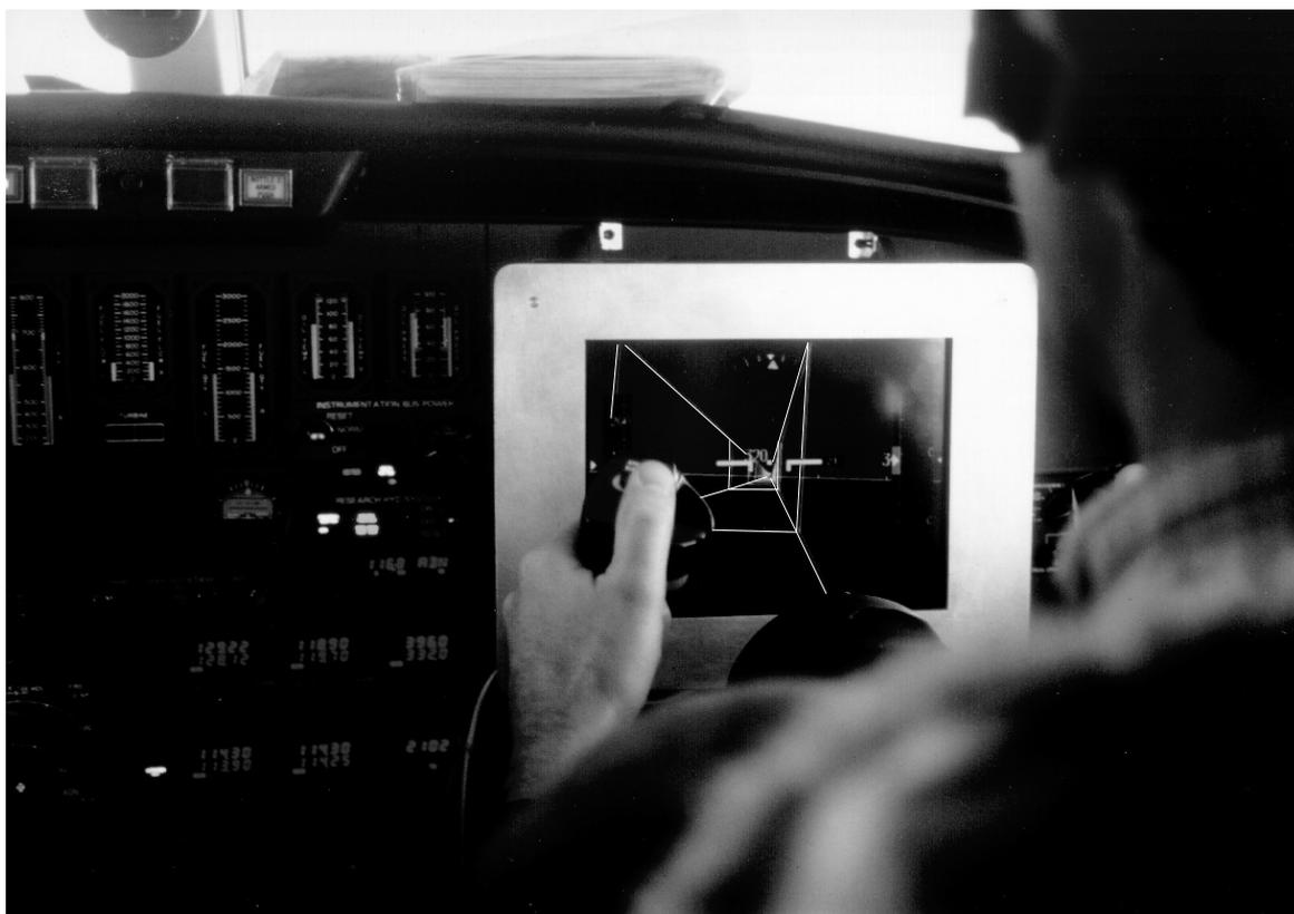
**Fig. 7.68.** *In-flight test of the perspective flightpath display on December 19, 1994. The pilot has to remain inside the tunnel. The presentation of the flightpath has been accentuated.*
