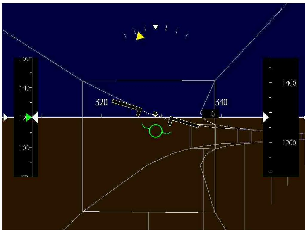
**Fig. 6.20.** *Outside-in version of the display format presented in Fig. 6.14 for a situation in which the roll angle is approximately 17 degrees.*
