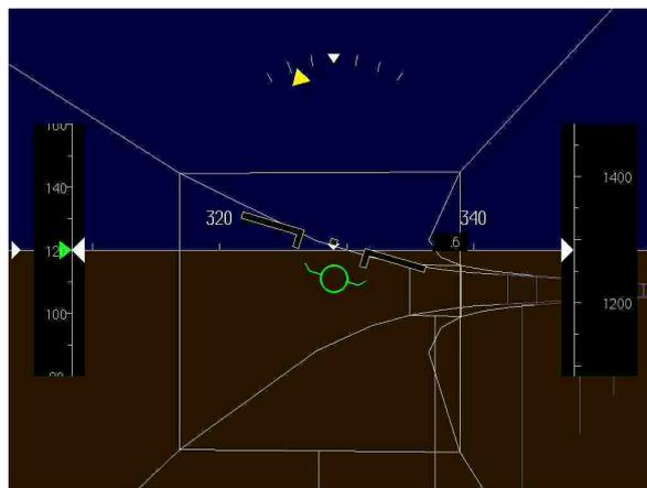
**Fig. 7.3.** *Outside-in frame of reference. In this frame of reference the horizon is fixed and the aircraft symbol moves the same way as the real aircraft when seen from a position behind it.*
