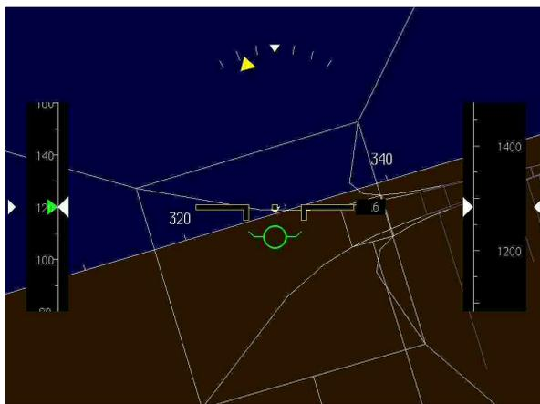
**Fig. 7.2.** *Inside-out frame of reference. In this frame of reference the aircraft symbol is fixed and the horizon rotates and translates the same way as the horizon the pilot perceives when looking through the windshield.*
