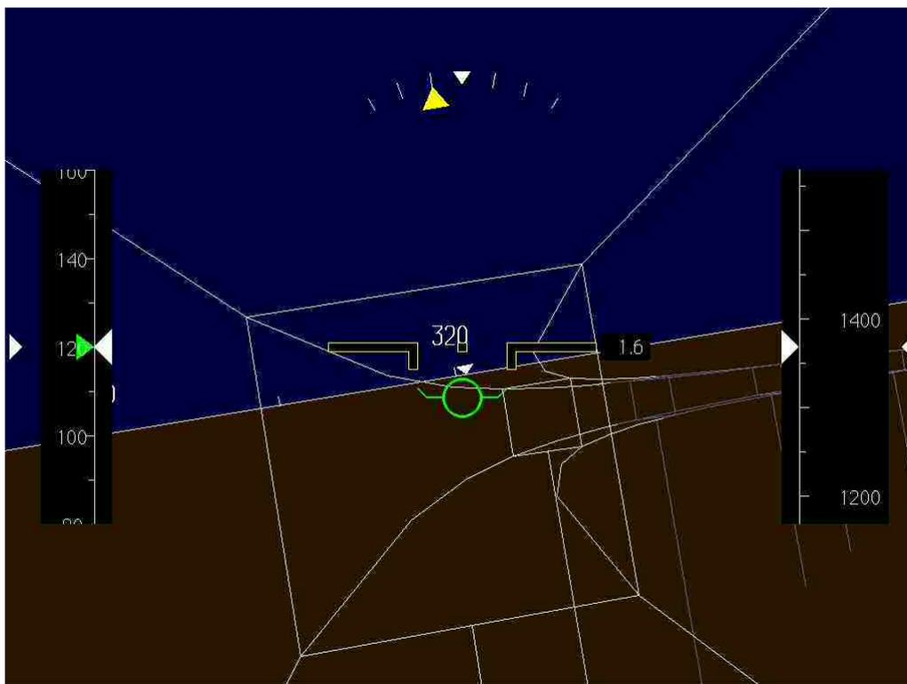
**Fig. 6.14.** *Basic display format in the flightpath vector configuration with tape instruments for the presentation of altitude and velocity. The symbology is explained in Fig. 6.13.*
