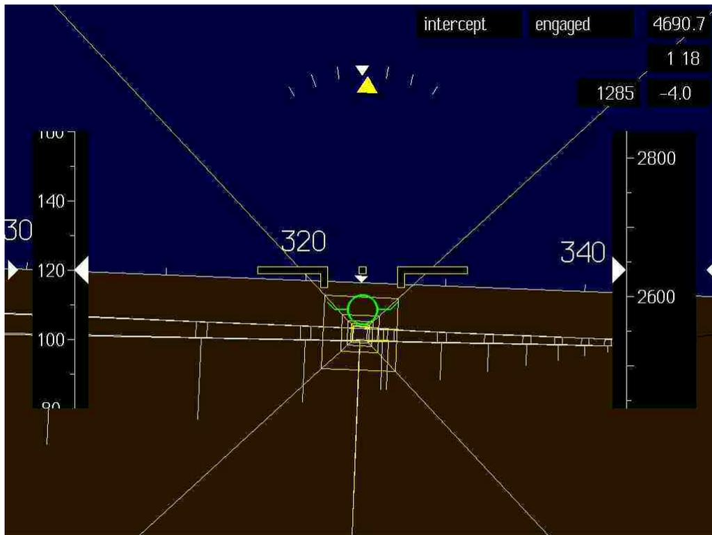
**Fig. 6.23.** *Intercept tunnel towards the approach path. The symbology is explained in Fig. 6.25.*
