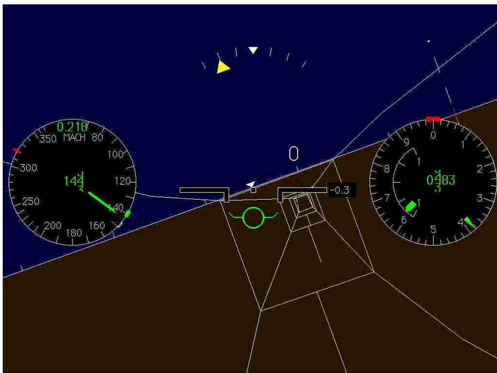
**Fig. 6.15.** *Basic display format in the flightpath vector configuration with dial instruments for the presentation of altitude and velocity.*
