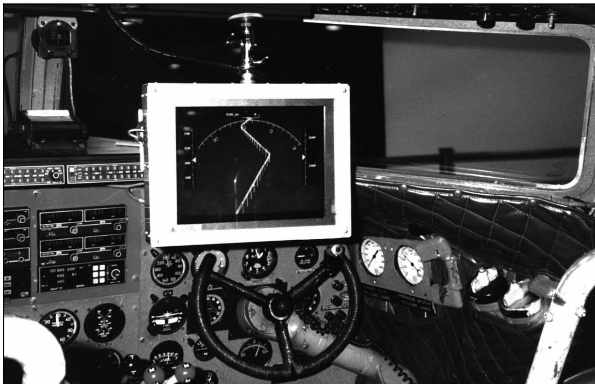
**Fig. 7.69.** *Display system installed in the DC-3 laboratory aircraft of the Avionics Engineering Center of Ohio University in Athens.*
